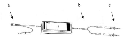
a. Output Cable The output BNC connector and the auxiliary grounding terminal are connected to the oscilloscope.
