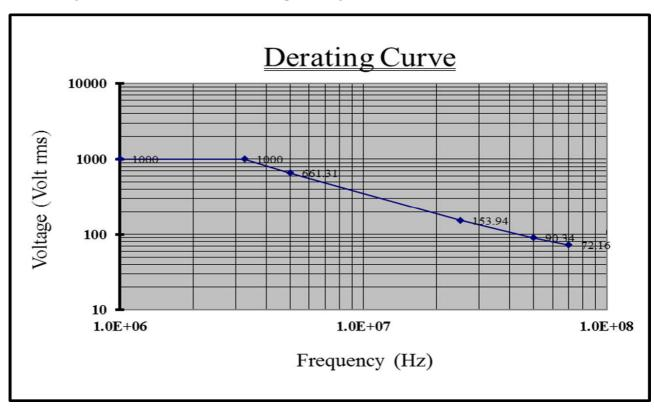
The derating curve of the absolute maximum input voltage in common mode is shown as follows;
